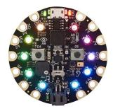
This is one of the boards we used for the Spark workshop at MIT. It has 10 colorful NeoPixel LEDs, as well as two buttons, a tilt sensor, a built-in speaker, and IR remote receiver, and many other features. You can connect external servo motors or NeoPixel strips to the pads around the edge of the board.
