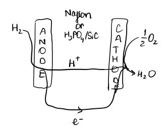
GDE is typically made up of Pt/C on carbon cloth.
