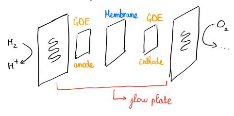
H2/O2 just cell can operate in acid or basic conditions
